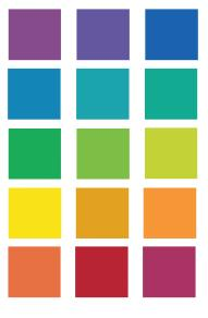
source spectrum that would render saturated colors well, and render unsaturated colors poorly. This important result shows that nothing is lost and everything is gained by only using saturated colors as our new sample set. Therefore, CQS uses fifteen saturated colors chosen to be evenly spaced across the entire visible spectrum.
