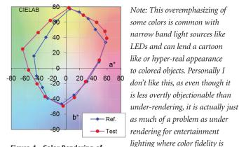
Figure 4 - Color Rendering of RGB LED with CRI of 67
