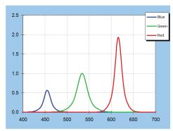
Figure 3 - Spectra of RGB LED with CRI of 67
