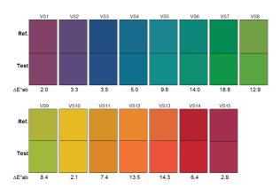
Figure 9 - CQS samples under RGB LEDs at 455nm, 534nm and 616nm
