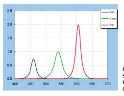
Figure 1 -Spectra of RGB LED with CRI of 81
